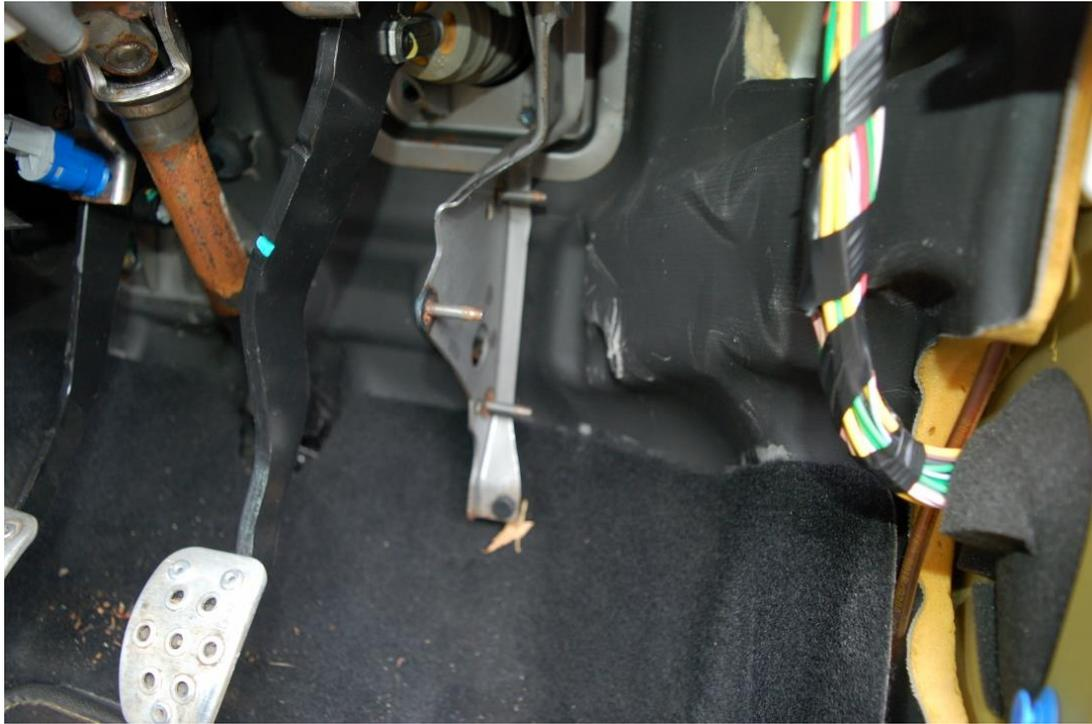
Trim a small section of sound deadening out from around the bulkhead grommet shown in the photos below.
