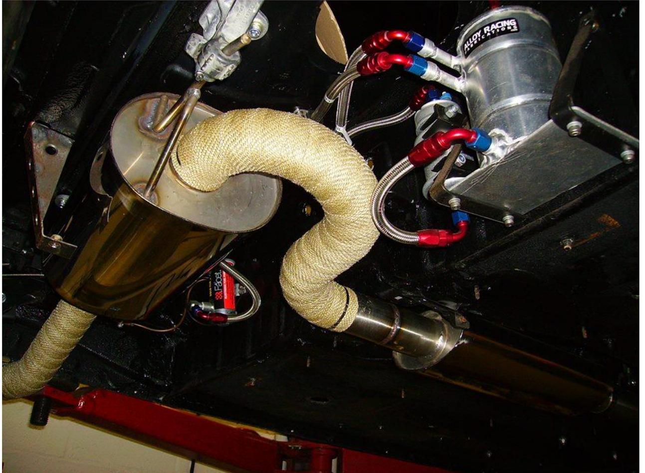
**Ensure that the connection pipes are correctly mounted and do not pull tight with engine movement.** Spigot-ended fuel rails are only 8mm diameter under the hose - insufficient to restrain an engine without breaking!
