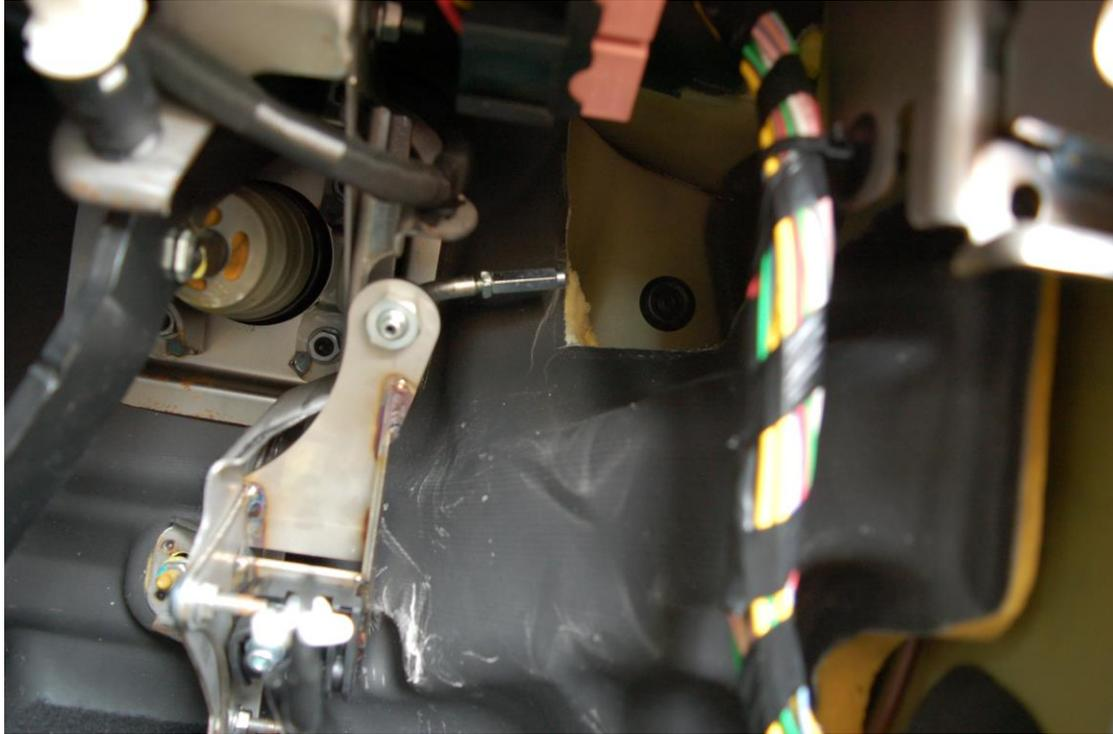
From the inside of the car pass the new cable through the clip, through the 90 degree fitting in the bracket, into the outer sheathing and through the bulkhead and push the clip into the pedal.
