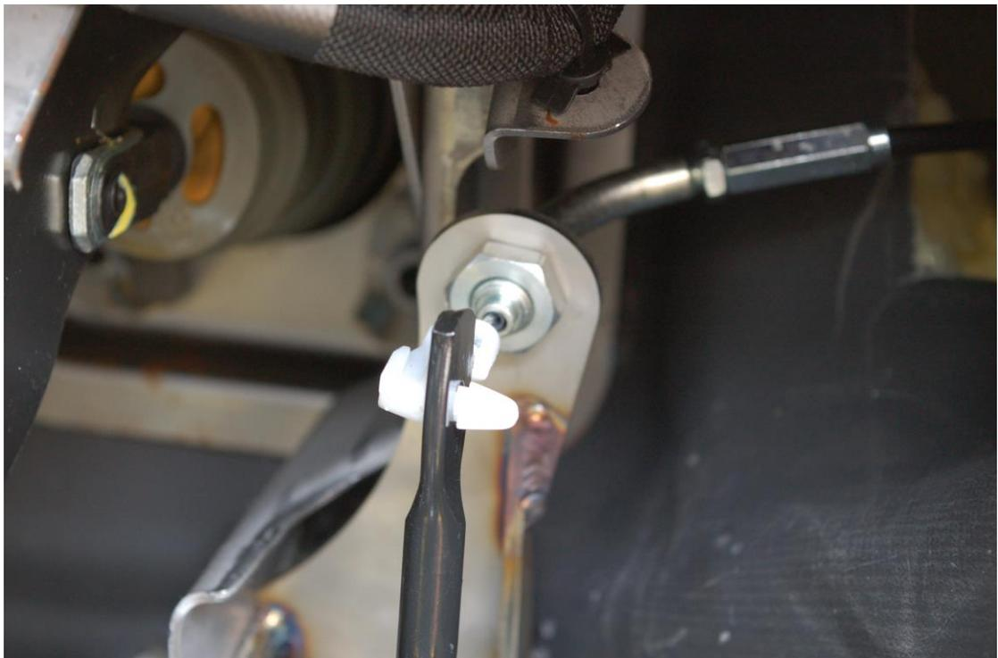
Fit the throttle cable end clamp into the base of the throttle quadrant.
